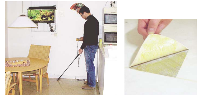
FIGURE 9. An inventory carried out before rebuilding will reveal critical construction solutions and faulty functions that could constitute risks for the indoor environment and the air quality. This means that major problems can be discovered in time, with great cost savings as a result. The photograph shows moisture measurements being carried out with a moisture meter, to find floor areas with excess moisture content. If floor coverings are placed on top of damp floors, chemical substances could be released and affect the quality of the air.
