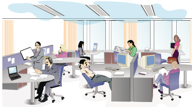
FIGURE 10. Active climate beams in an open plan office.
