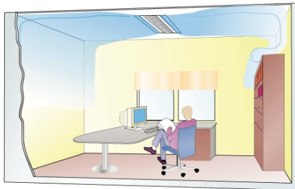
FIGURE 7. An active climate beam positioned at right angles to an external wall.
