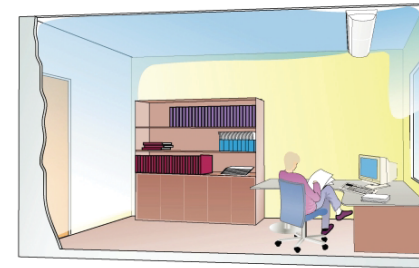
FIGURE 8. An active climate beam placed parallel to an external wall.
