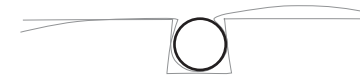
FIGURE 4. An example of how an airtight join between two sheets of plastic can be achieved by placing the overlapping areas over a U-shaped metal jointing strip and pressing the sheets together using plastic tubing.
