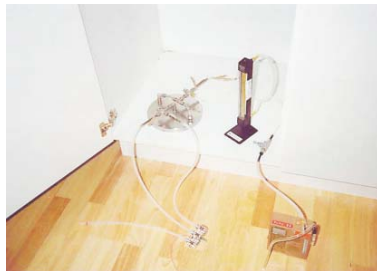
FIGURE 3. Fulfilment of functional requirements stipulated for the indoor climate must be verified by carrying out appropriate measurements. The picture shows equipment for measuring emissions from furnishings.
