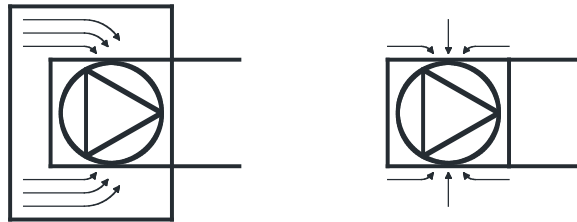
FIGURE 4. Air flow patterns around an enclosed and unenclosed centrifugal fan with double intakes.
