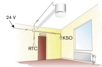
FIGURE 13. An active ATD with an external room thermostat and sequentially controlled radiator valves.
