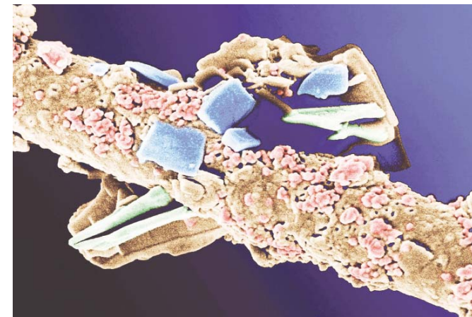
FIGURE 5. Nanoparticles on a strand of filter fibre. © LENNART NILSSON PHOTOGRAPHY AB/CAMFIL AB
