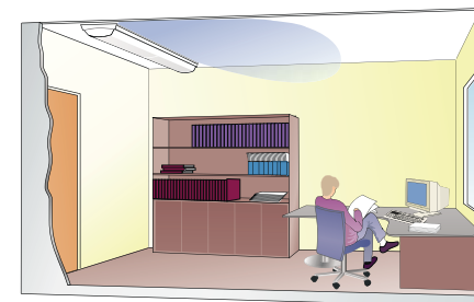
FIGURE 9. An active climate beam placed close to a corridor wall.
