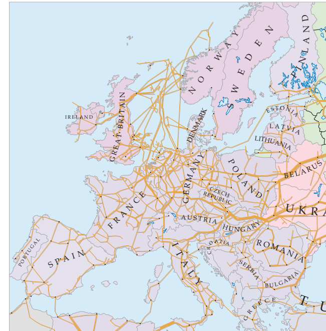
FIGURE 3. Europe’s existing and planned gas transmission networks. Illustration: GAZPROM in questions and answers ( http://eng.gazpromquestions.ru/ ), GAZPROM.
