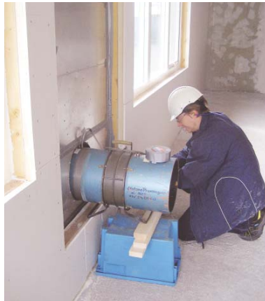
FIGURE 6. The airtightness of the building envelope can be easily assessed by carrying out airtightness tests. When these tests are carried out there is also often a search for leaks, so they can be identified and sealed. If the degree of airtightness is insufficient, this can affect the ventilation, the quality of the air, moisture protection measures, thermal comfort and energy use.
